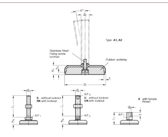
$\begin{array}{l} A/F1 = 17 \\ d1 &= 100 \\ d2 &= M10 \\ h1 &= 20 \\ h2 &= 6 \\ h3 &= 28 \\ l1 &= 60 \\ s &= 3 \end{array}$
